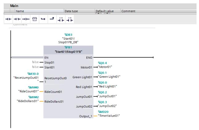
Function block shows more information regarding the programming inside, and as users, we can monitor the data without going to the function block itself. Because of that reason, function blocks are easier to use for more complex programming while function call can be used for quick and frequent functions. In our case, both work fine.
